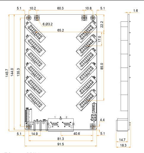
Tolerance: ±0.3 Unit: mm
