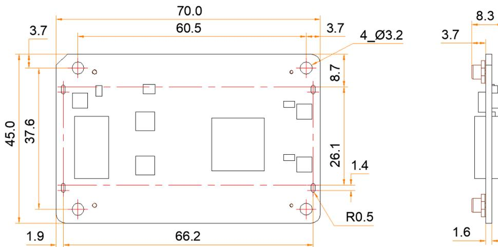
Tolerance:  $\pm 0.3$  Unit: mm
